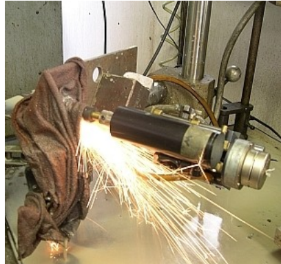
Job: EDM 5/8" hole in 1/4 plate horizontally using magnetic base. Electrode: Graphite .610" OD, .460" ID Time= 6 minutes unattended Notice core in last photo.
