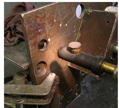
Job: EDM 5/8" hole in 1/4 plate horizontally using magnetic base. Electrode: Graphite .610" OD, .460" ID Time= 6 minutes unattended Notice core in last photo.
