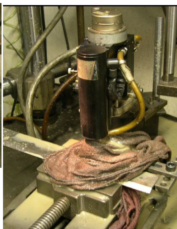
Job: EDM 5/8" hole in 1/4 plate horizontally using magnetic base. Electrode: Graphite .610" OD, .460" ID Time= 6 minutes unattended Notice core in last photo.
