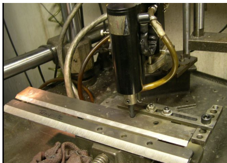
Job: EDM 5/8" hole in 1/4 plate horizontally using magnetic base. Electrode: Graphite .610" OD, .460" ID Time= 6 minutes unattended Notice core in last photo.
