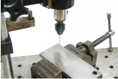
EDM .028" hole through 1/4 Stainless steel Electrode: .024 Brass tubing Time 4 minutes
