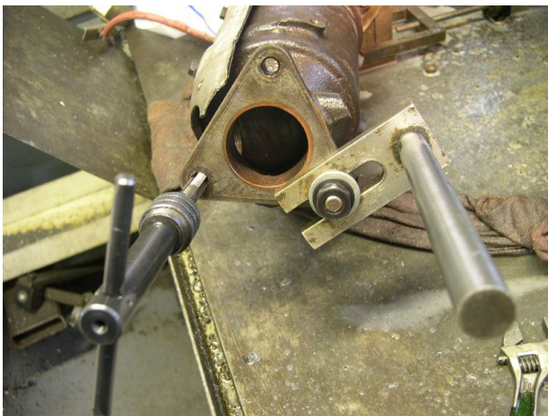
Shows setup and cleanup of threads with tap.
