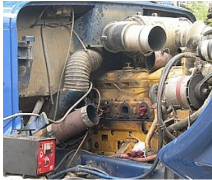
Shows EDM machine setup on diesel truck motor to remove an exhaust manifold stud broken off in cylinder head.
