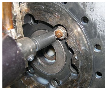
Job: Broken stud in crankshaft end plate. Engine is in vehicle and on a lift with transmission and flywheel removed (photo 1). Machine is set up using a neighbor threaded hole in crankshaft (photo 2). Hole after EDM work and before picking out remaining thread sleeve Electrode: Graphite tube 10 mm stud 20 mm deep Time: 12 minutes. Last photo shows stud removed and ready to pick out remainder of thread sleeve .
